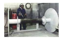
Metal sprayed coatings being applied to winch components for use in corrosive salt-water environment.
