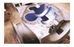
This badly corroded, Split Casing Circulating Pump was completely refurbished using Ceramic Metal. Overall coating provided erosion corrosion protection.
